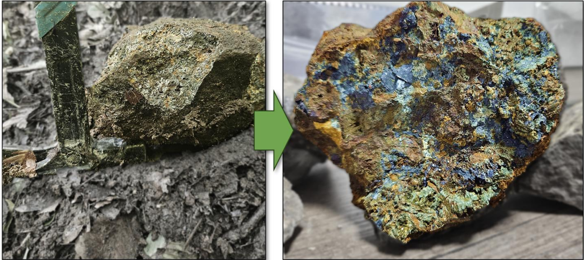
Figure 4: Gradina Prospect, mineralised float sample near old workings (photo shows original sample split open), containing approximately 15-20% galena+sphalerite. Refer to Table 1 Sample ID GRRC001 for assay results and Table 2 for Visual Observations.
