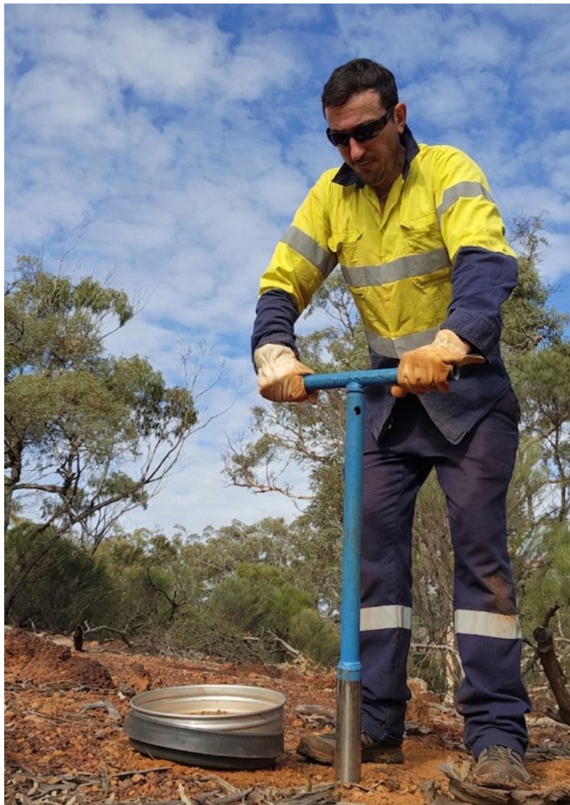
Figure 7. Hand-auger soil sampling at the Watheroo prospect.
