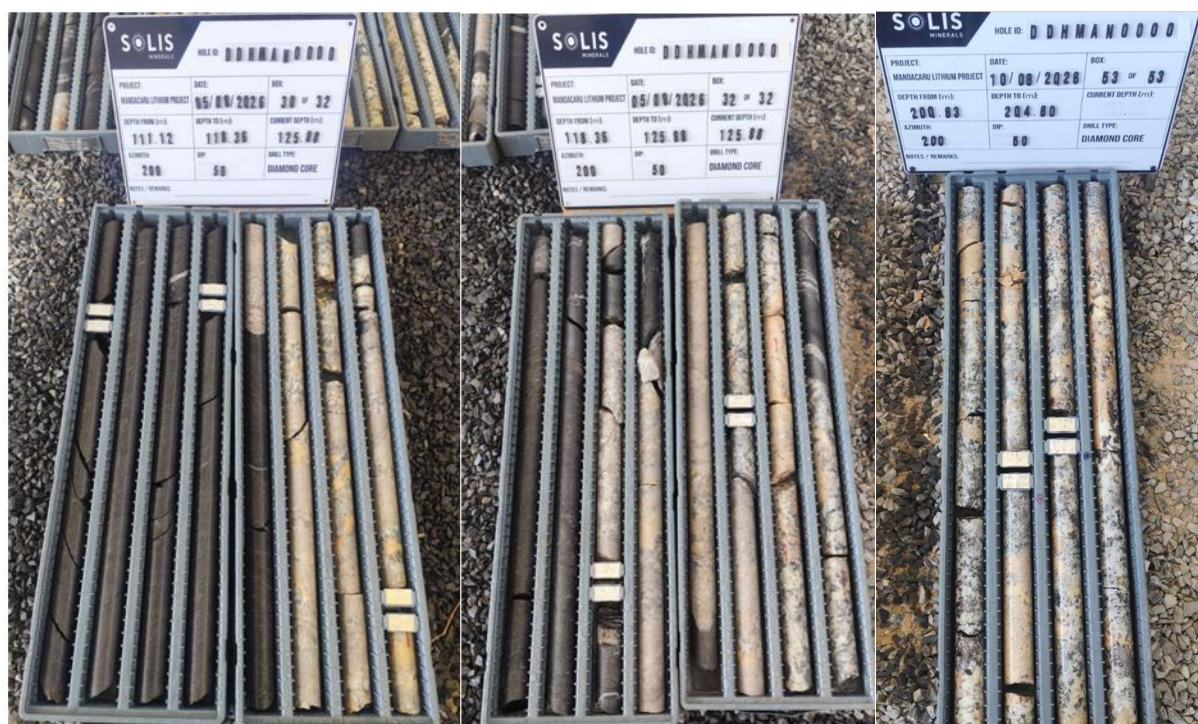
Figure 2: Core from completed drill-hole PDH-05. Visuals should never be considered a proxy or substitute for laboratory analyses where concentrations or grades are the factor of principal economic interest. Visual estimates also potentially provide no information regarding impurities or deleterious physical properties relevant to valuations.
