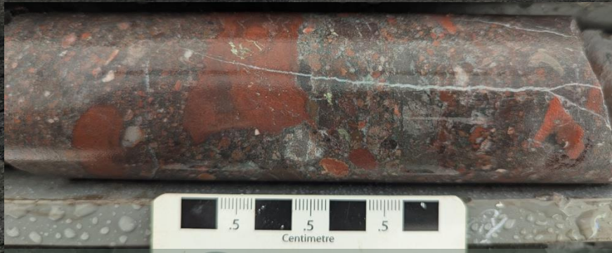
Photograph of disseminated, fine grained chalcopyrite within the basal conglomerate at the contact of the Rae Group and underlying Husky Creek Formation in drillhole SED26002
