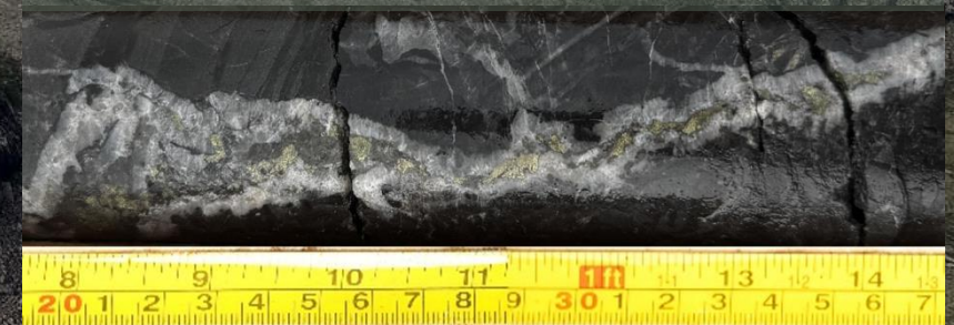
Example of chalcopyrite-bornite hosting quartz-carbonate veining in STK25001 between 181.30 and 181.52m downhole. Core diameter is NQ2.
