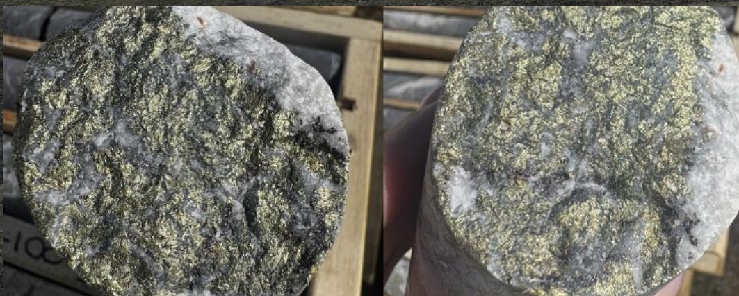
Chalcopyrite-bornite-quartz-carbonate veining below the base of the sedimentary structure in STK25001 at 291.4m that returned assays of 14.95% Cu & 0.51g/t Au. Core diameter is NQ2
