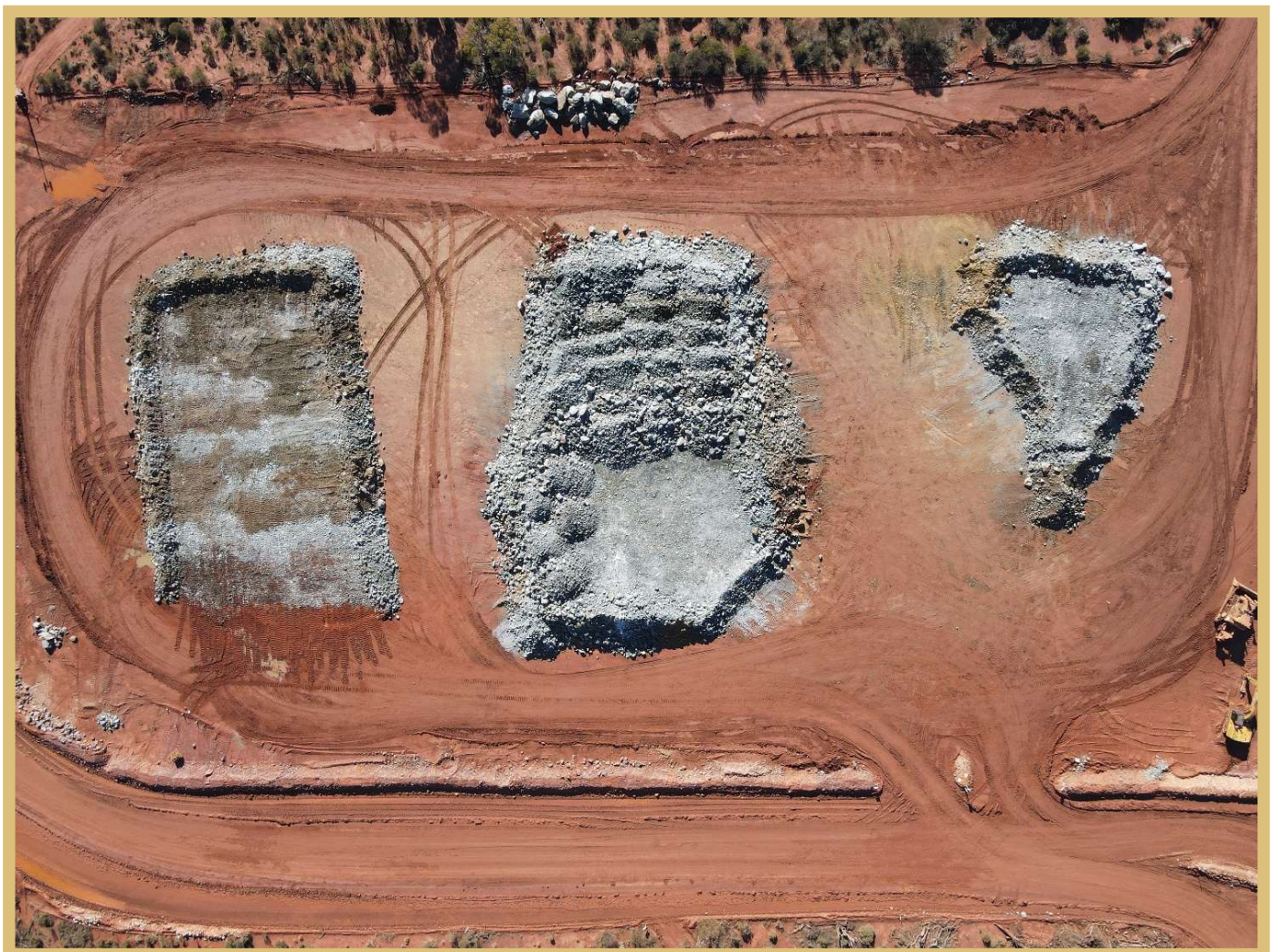
Figure 3: The Mine Ore Pad – where certified parcels are placed by the Company and paid for by SIGM under the OPA.
