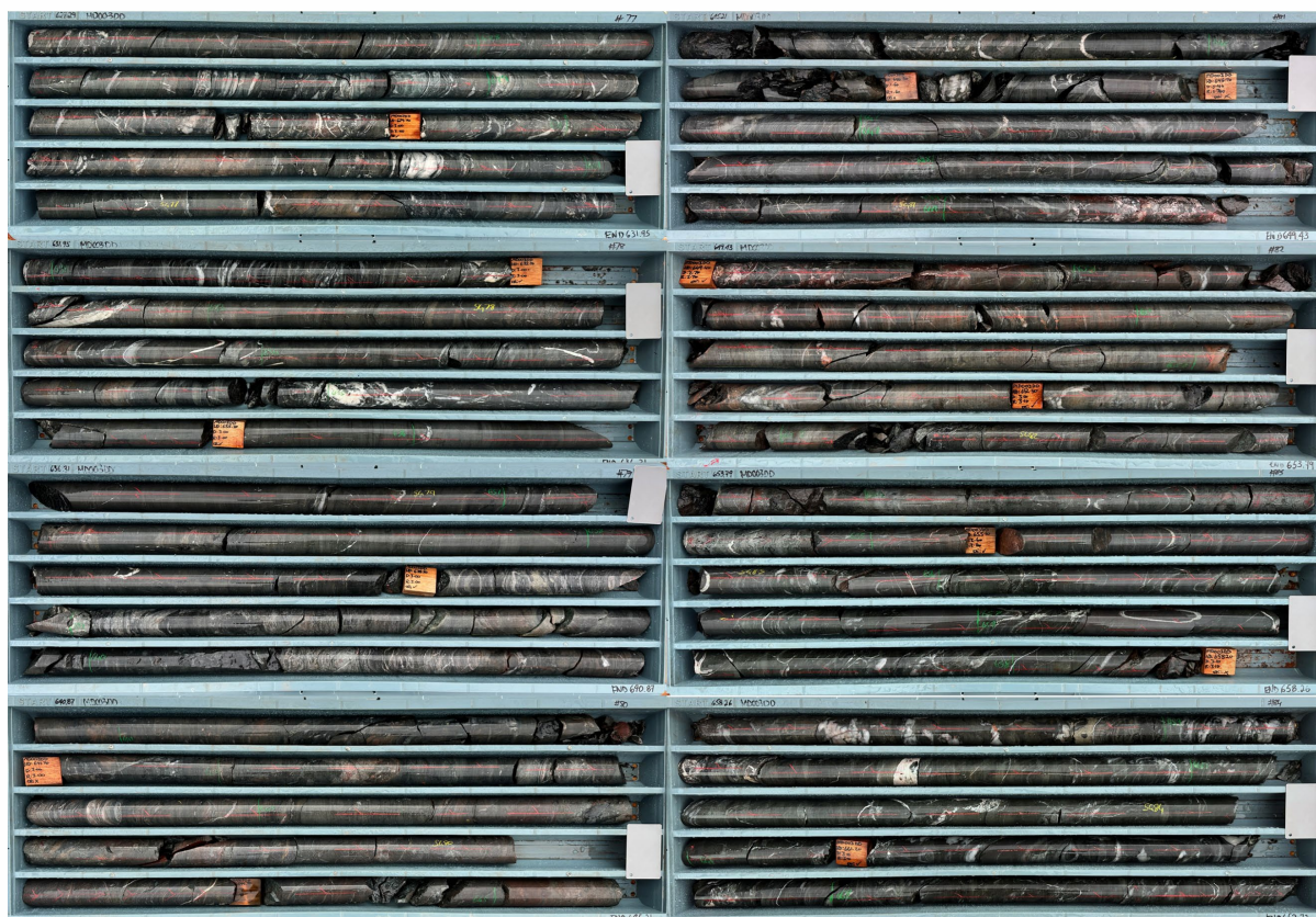
Figure 3: Wet core photography, MD003DD 627.29–662.72 m (trays 77–84, NQ3 core, 45.0 mm diameter). The interval contains two zones of intense quartz-carbonate stockwork veining and brecciation — 627–636 m, most intense at 630–631 m, and 645–663 m, where vein intensity increases progressively downhole and remains elevated at the base of the imaged interval. These are separated by a finely laminated unit at 636–645 m of lower vein abundance which nonetheless hosts localised massive pyrite, indicating that sulphide distribution is not controlled by vein intensity alone. Disseminated and fracture-controlled pyrite with trace chalcopyrite occurs throughout the interval, averaging approximately 0.5% total sulphide abundance excluding the discrete massive sulphide zones. Assay results are expected by the end of September 2026.
