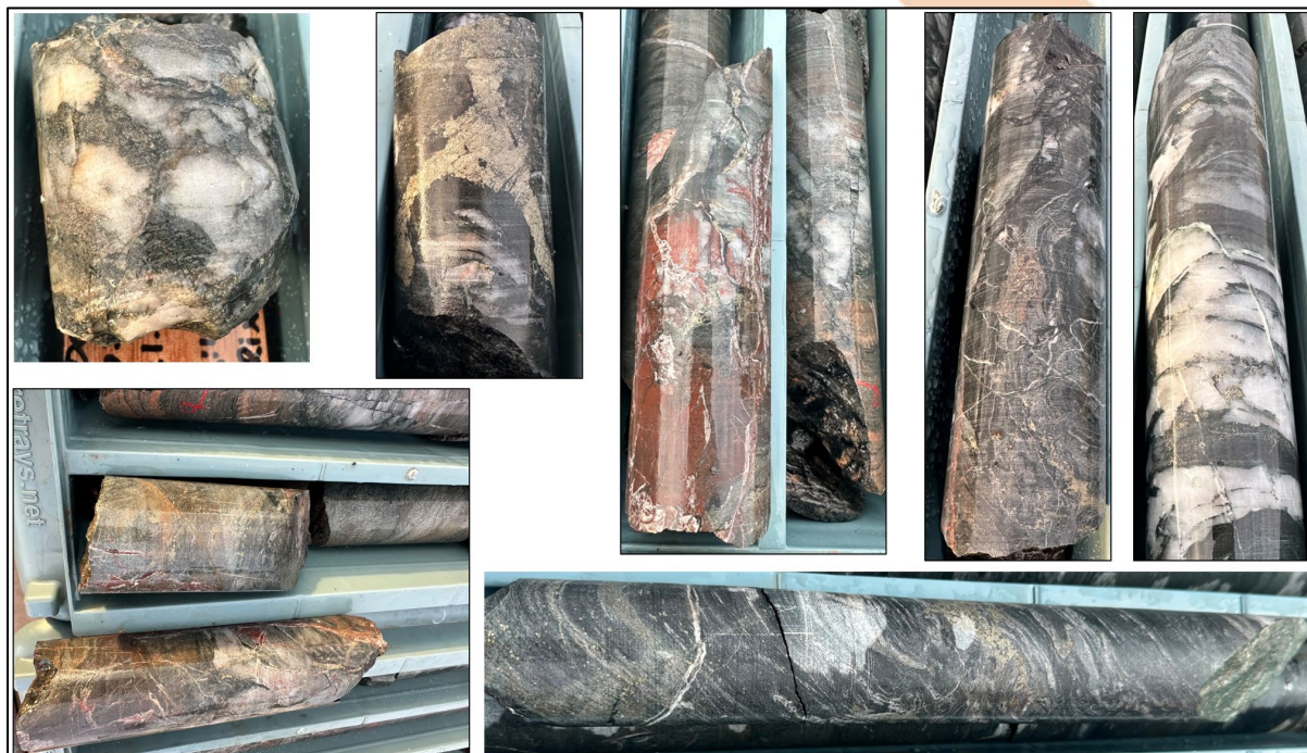
Figure 4: Selected alteration textures, altered basement sequence (gneissic metasediment and metamorphosed banded iron formation), MD003DD (627.29–662.72 m NQ3 core, 45.0 mm diameter), illustrating quartz-carbonate vein breccia, cm-scale veins of massive pyrite>>chalcopyrite, silica-carbonate and hematite alteration, folded and transposed banding, and cross-cutting carbonate, quartz-carbonate and quartz veining. Images are selected to illustrate complex textural variability and are not representative of the interval; assays are pending and no mineralisation is implied. Per figure 3, the entire interval 627.29–662.72 m has disseminated and fracture-controlled pyrite and traces of chalcopyrite averaging 0.5% total sulphide abundance.
