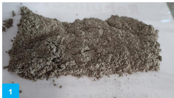
Figure 5: 1. Pulverised spent catalytic converter; 2. Conventional flowsheet for catalytic converter processing (Yakoumis, I., et al. 2021)
