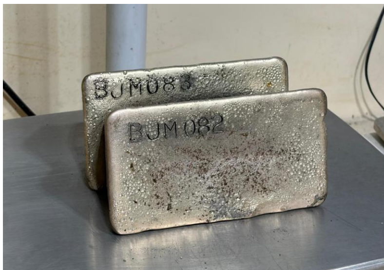
Figure 1: Elution doré bars BJM082 and BJM083, with a combined weight of approximately 593.8oz, produced during the 11 August 2026 smelt. The two bars form part of the three-bar BJM082–BJM084 campaign, which produced a combined 861.3oz of doré. Official refinery assay and outturn are pending
