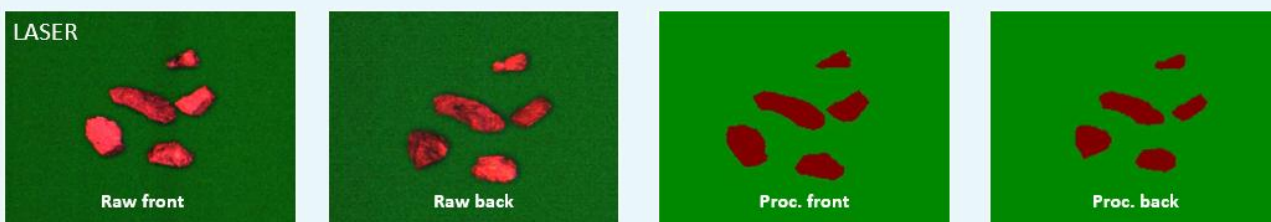
Figure 3 Ore sorting of various metallurgical sample types from Blue Bell by TOMRA. Both Laser and XRT Technology clearly differentiates between ore and waste types
