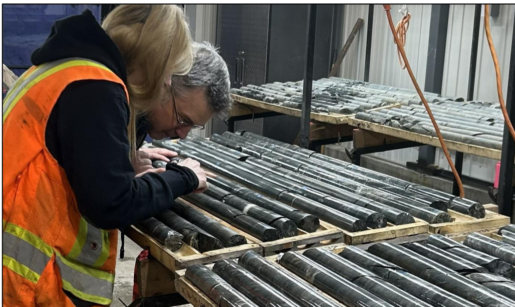
Figure 1 - Rouyn drill core being studied appraised prior to dispatch for assaying
