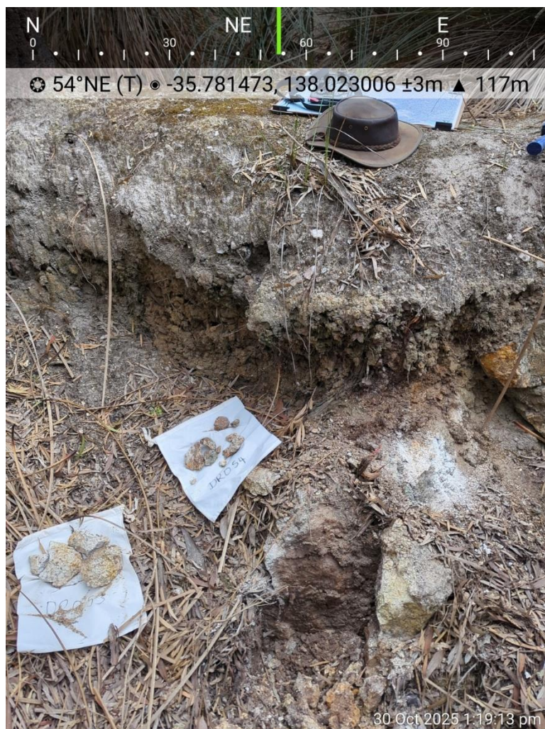
Figure 4 – Sample site of highly anomalous DR053 and DR054 in a small pit with ~50cm of soil overlying weathered outcrop
