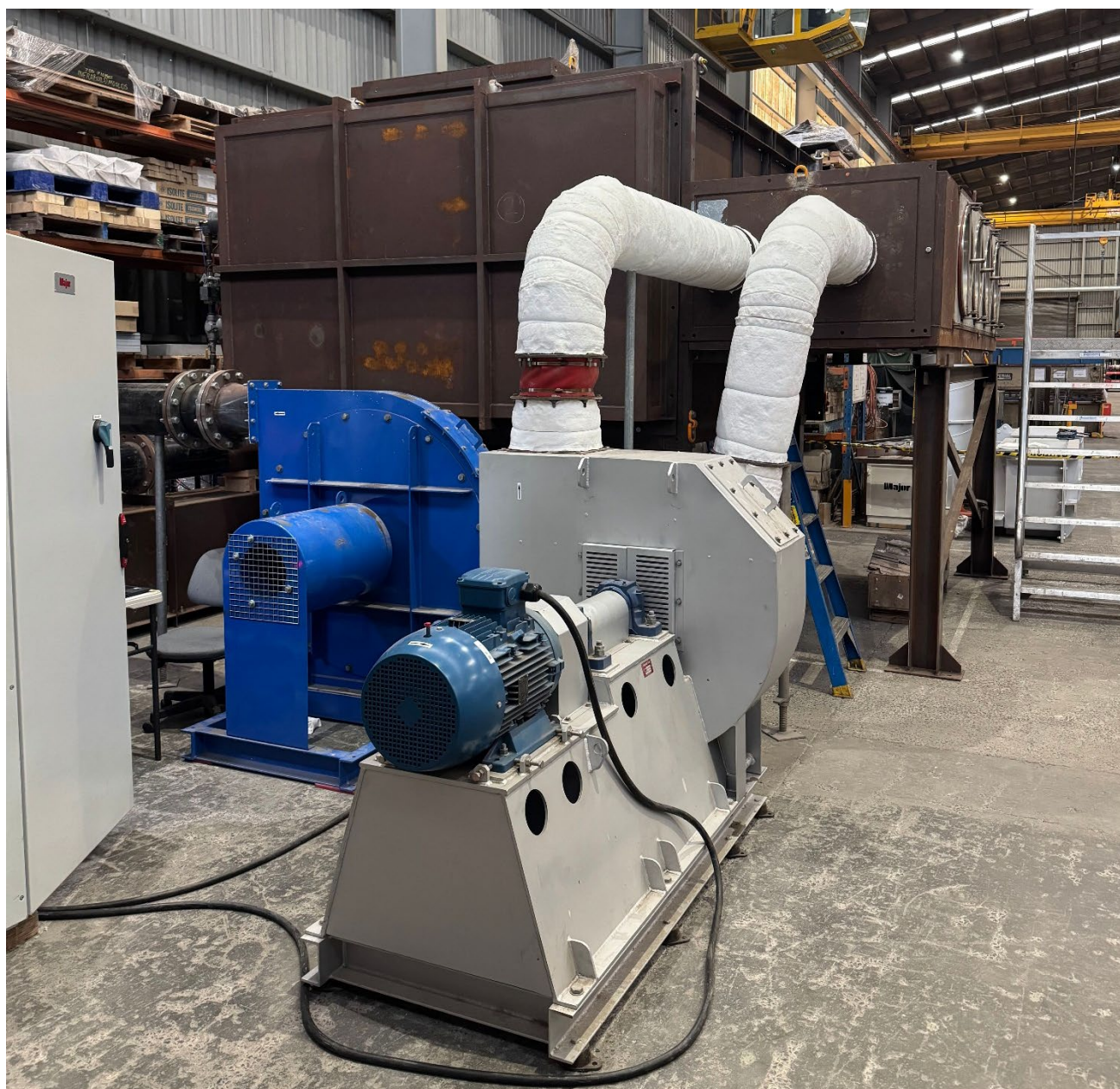
Prototype furnace test and successful validation of retort pier design at 1,180 degrees Celsius
