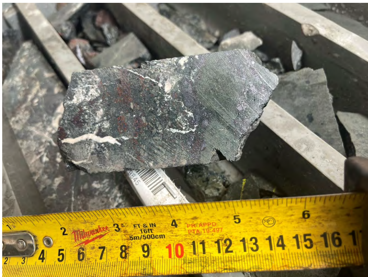
Figure 5 - Photograph of halved NQ2 diameter core showing mixed chalcocite and bornite mineralisation in the chlorite breccia zone at 45.5m in DAN26026
