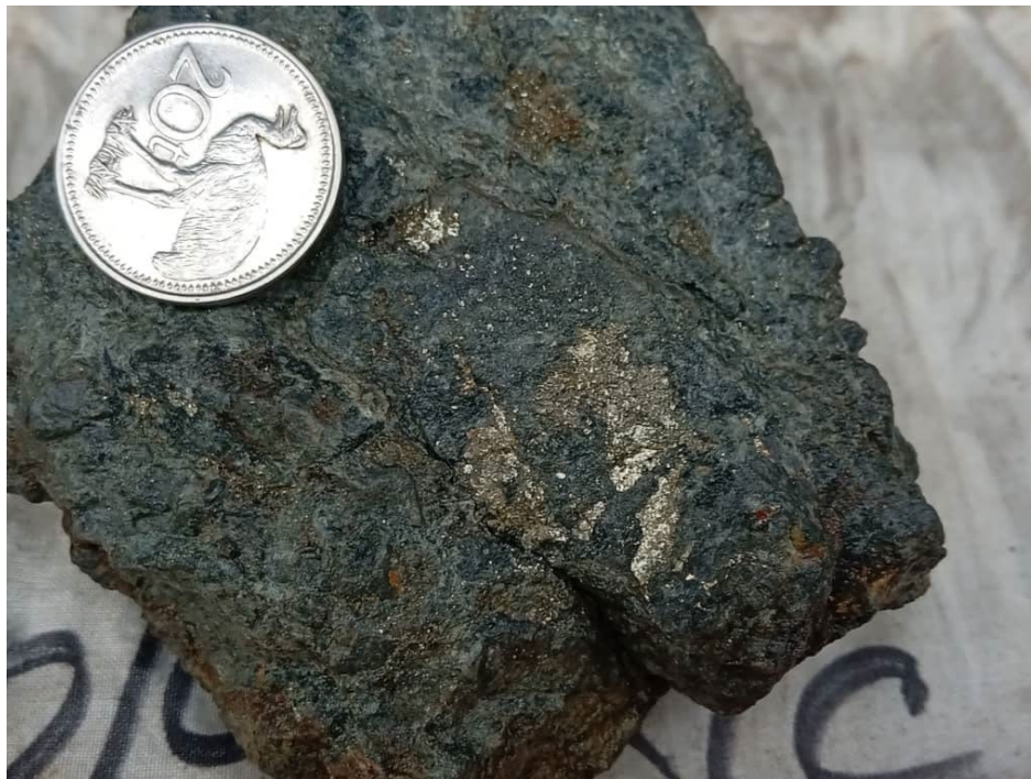
Figure 7: Outcrop Sample 702110 – Visible sulphides in breccia of andesitic volcanic sediment from North access track to Agadul. Visual estimate of sulphides 3% pyrite and 0.5% of fine chalcopyrite
