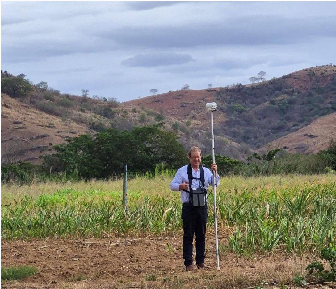
Figure 14: OZM CEO/MD in Brazil field testing and training with OZM ground magnetometer
