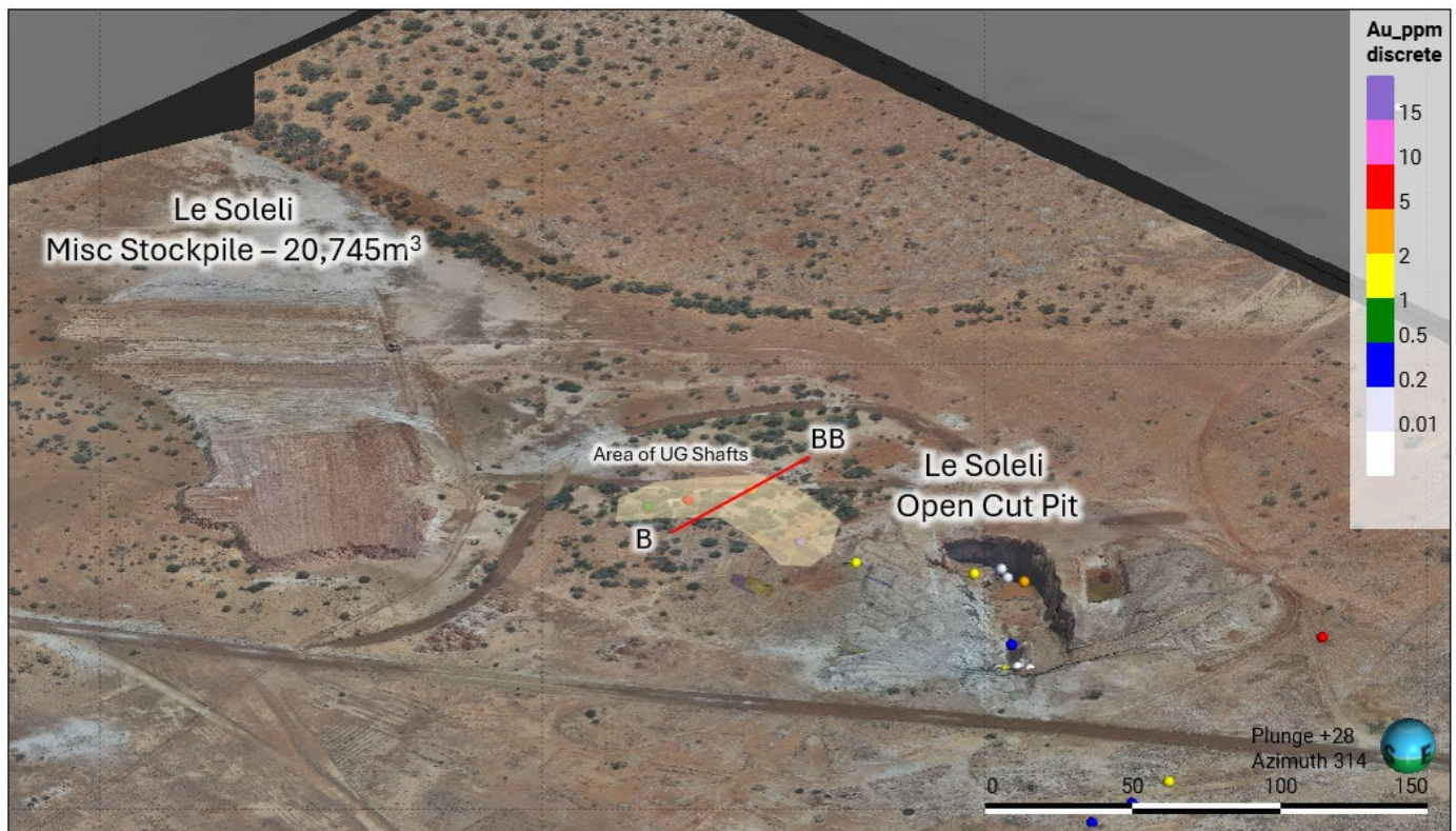
Figure 7. LiDAR imagery over Le Soleil's Historic Open cut pit and Miscellaneous Stockpile with historic grab samples looking northwest. *The coloured dots in Figure 7 are from Appendix A - Table 2 KRR ASX Announcement 18 May 2026*
