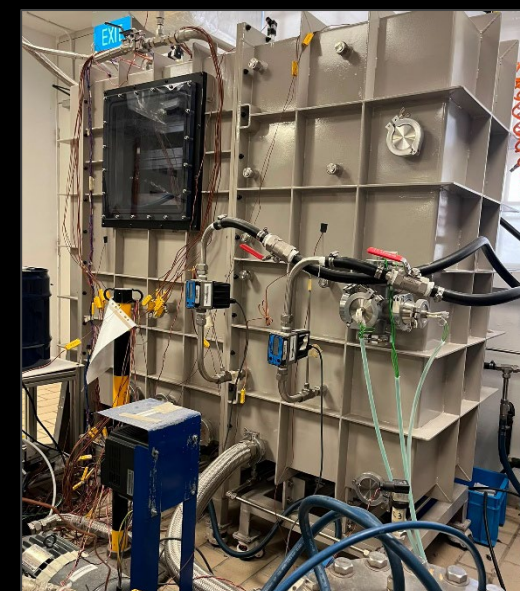
Lab-scale ~9 kW server rack chamber assembly.
