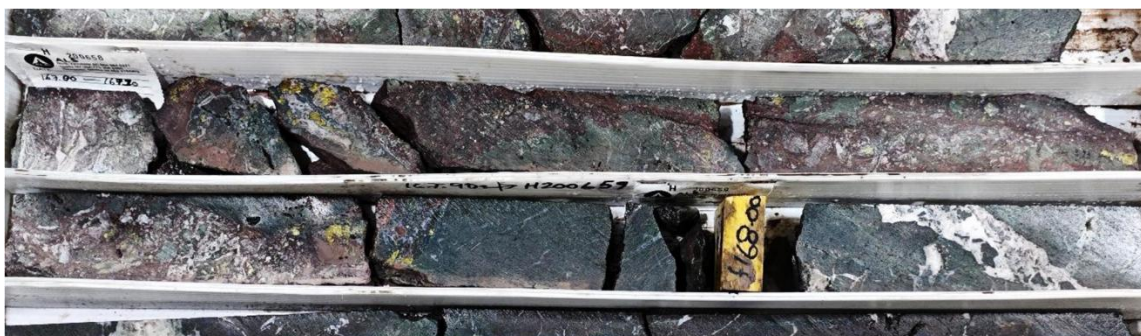
Figure 3. Section of cut core showing a complex breccia zone with hematite (brown), quartz (white) and the copper sulphide mineral chalcopyrite (yellow). Peak assay grades from this zone included 0.9m at 467g/t Ag, 0.6g/t Au, 1.4% Cu, 1.4% Pb & 2.1% Zn from 169m down hole. 2
