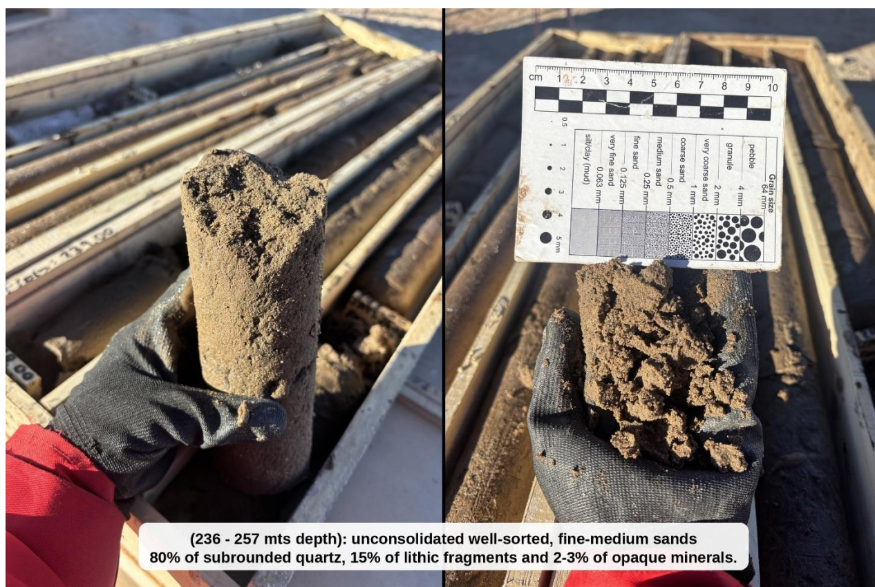
Figure 1. Well sorted sands encountered at 236-257m depth.
