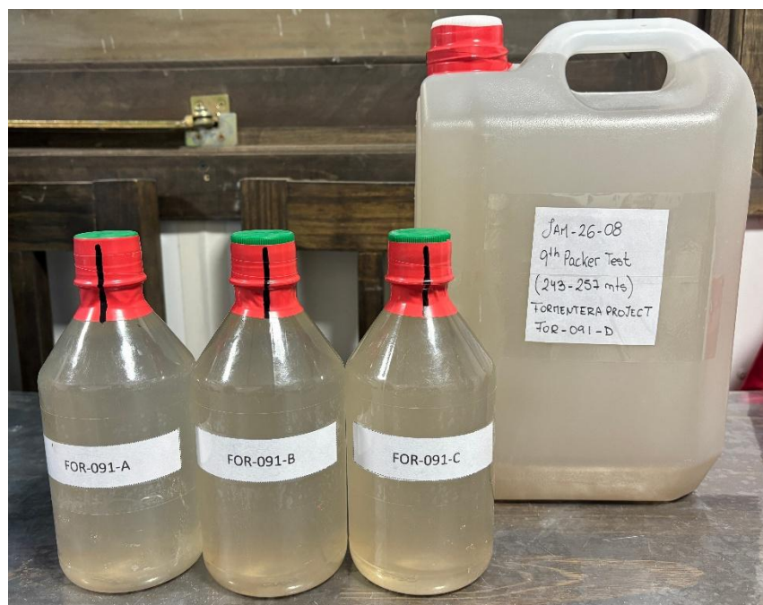
Figure 4. Brine Samples taken for lithium assay from packer test 9.
