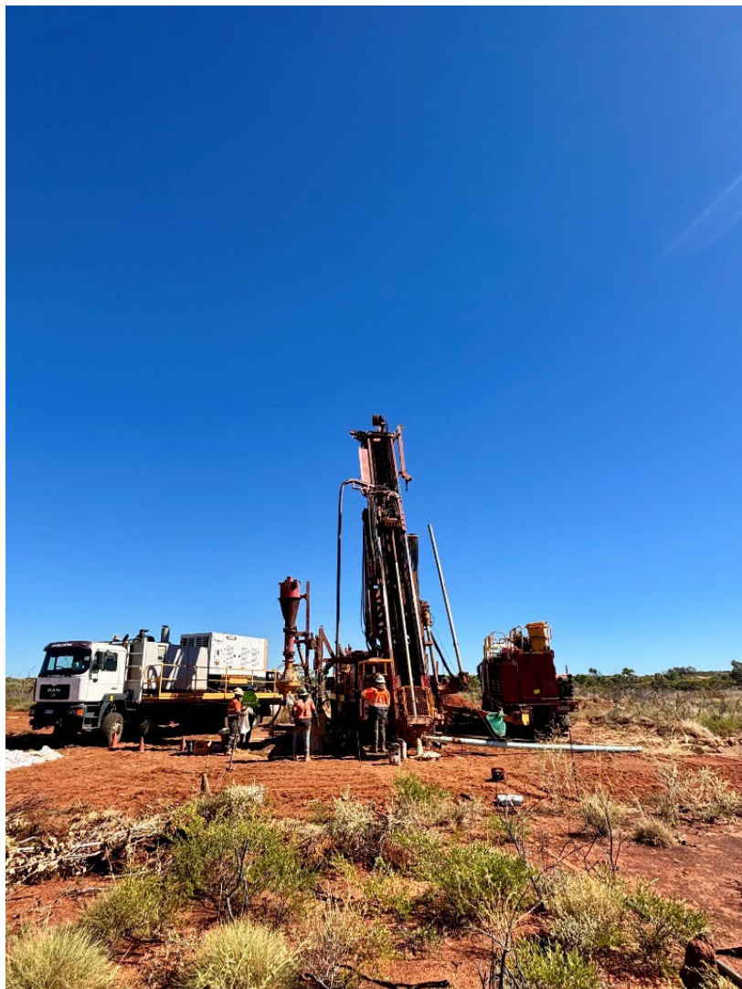
Figure 2: Bullion RC drill rig at Jims in June 2026.
