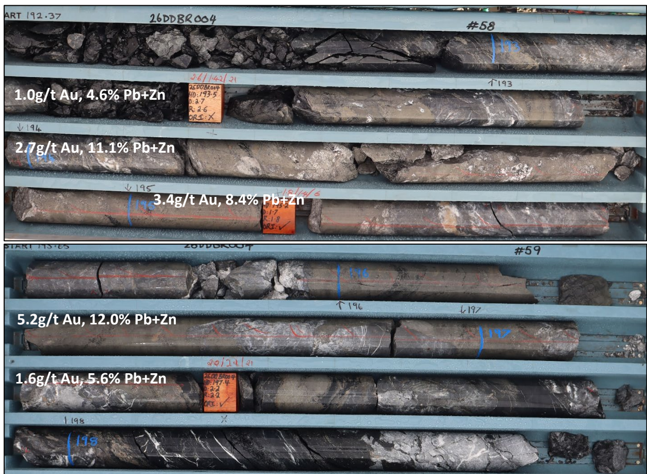
Figure 11: 26DDBR004 massive sulfide zone (brown), dominantly sphalerite and pyrite from 193m to 197.1m grading 5.1m at 2.7g/t Au & 8.3% Pb+Zn.
