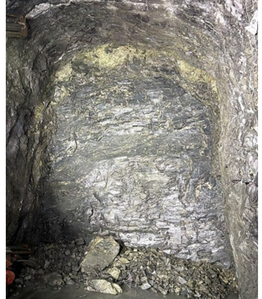
Development face passing through the J1 lens at Jericho, showing visible copper sulphide mineralisation. Face dimensions are approximately 5.5m wide by 7.5m high 2
