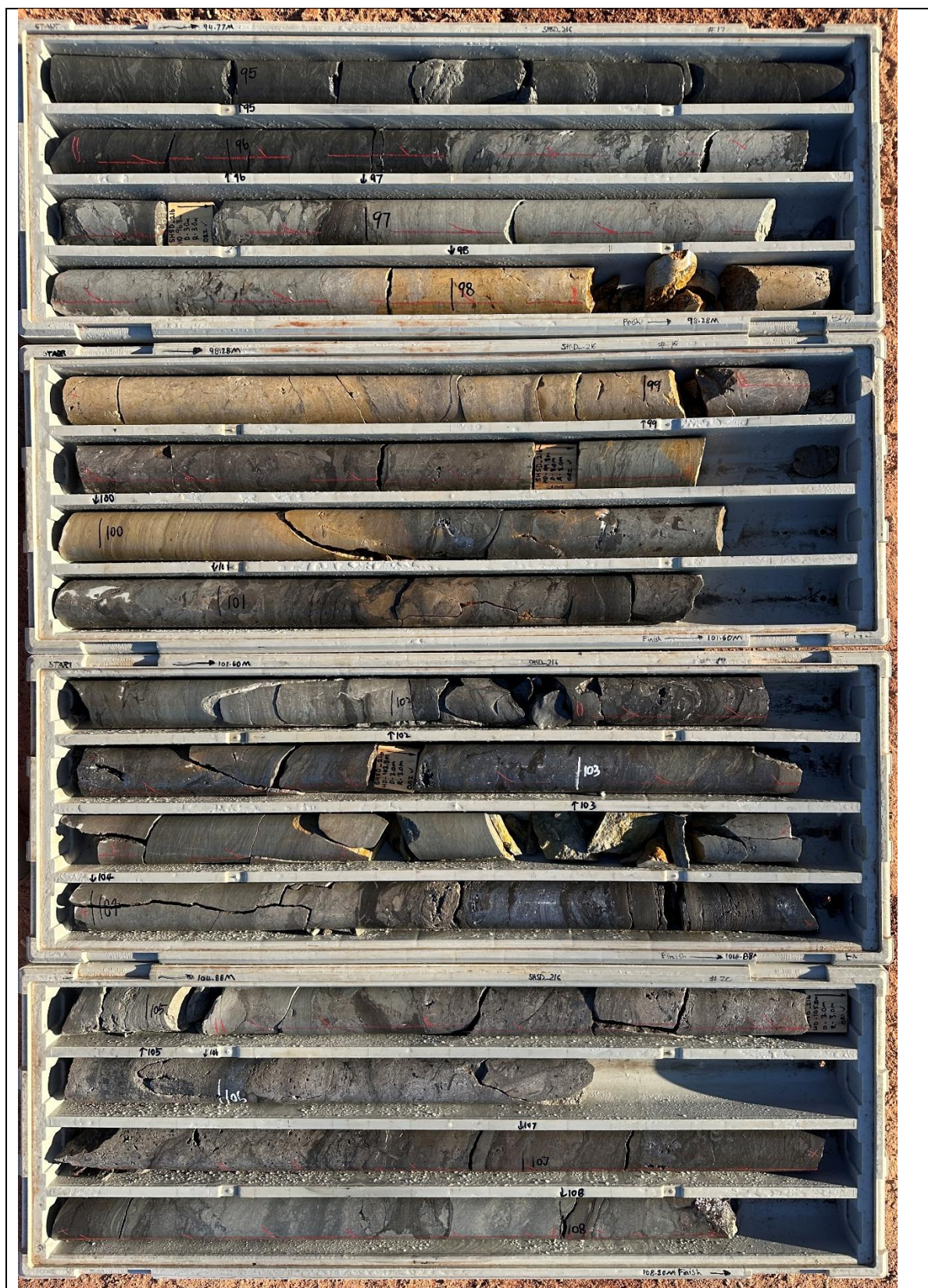
Figure 7: Photographs of drill core SHSD_214 and SHSD_216 illustrating the style of galena mineralisation intersected in SHSD_216 at Norton. Note: Table 1 provides detailed ore-sulphides estimates for the references drill intervals.
