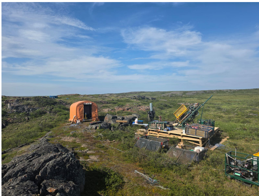
Figure 2: Photograph of reverse circulation drilling rig at JWS26001. Drillhole is targeting the historic “discovery zone” and will confirm the core of the known mineralisation
