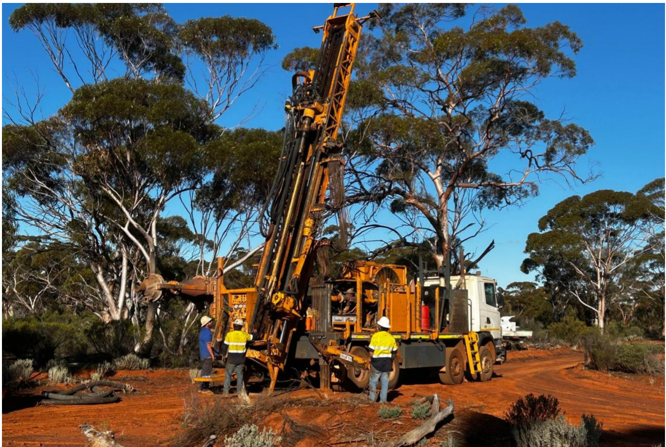
Figure 1: RC drilling in progress at the Mt Dimer Exploration Project (E77/2383)
