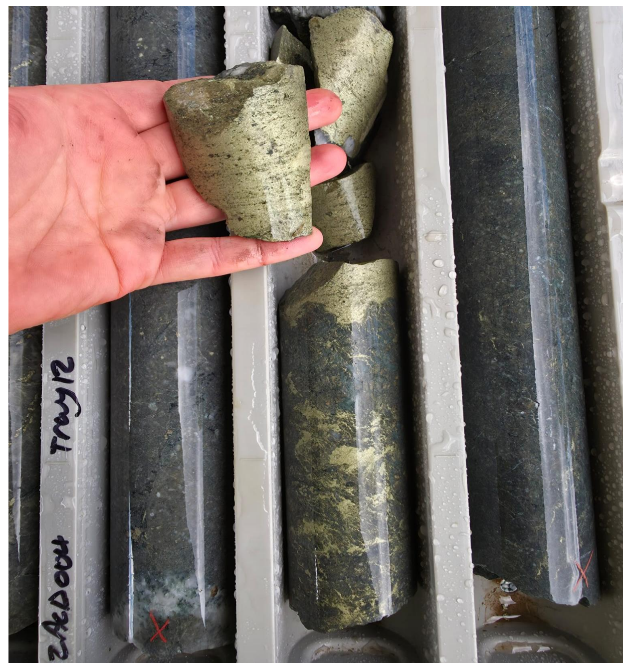
Monza hole MZACD004. Chalcopyrite and pyrite sulphide breccia within potassic altered monzodiorite porphyry. 0.99g/t Au & 4.1% Cu.
