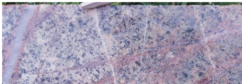
Photo 1 6 : 25CRC016, 670m – 671m 6 . 232ppm Mo, quartz – orthoclase - anhydrite fractured weak sericite altered monzodiorite
