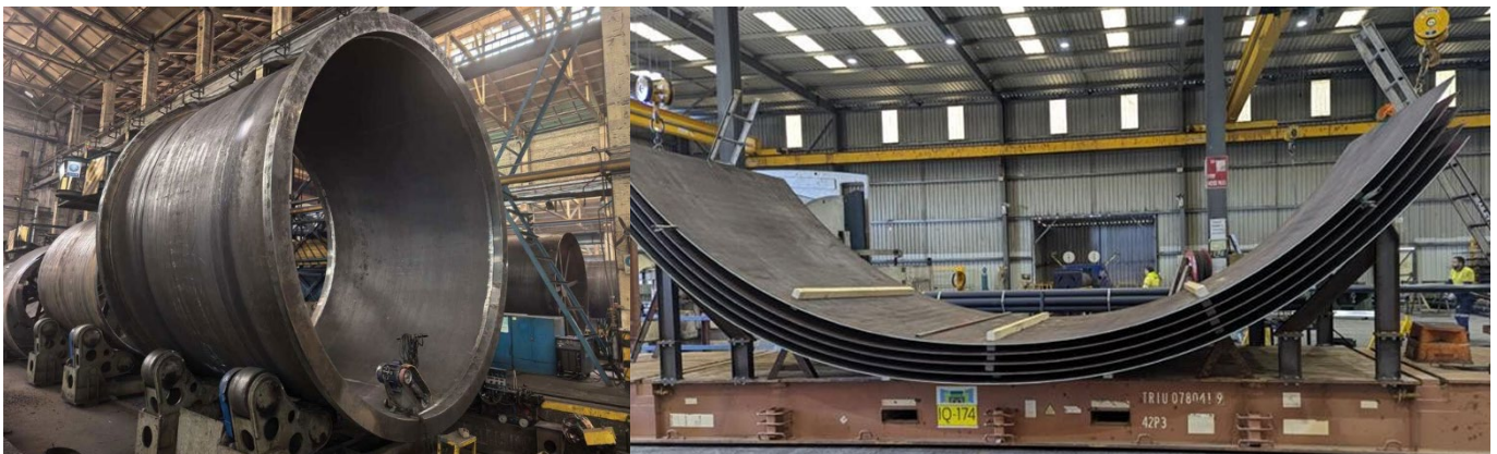
Figure 5 – Key processing plant component fabrication well advanced (ball mill shell on left, and CIL tank steel rolled on right)
