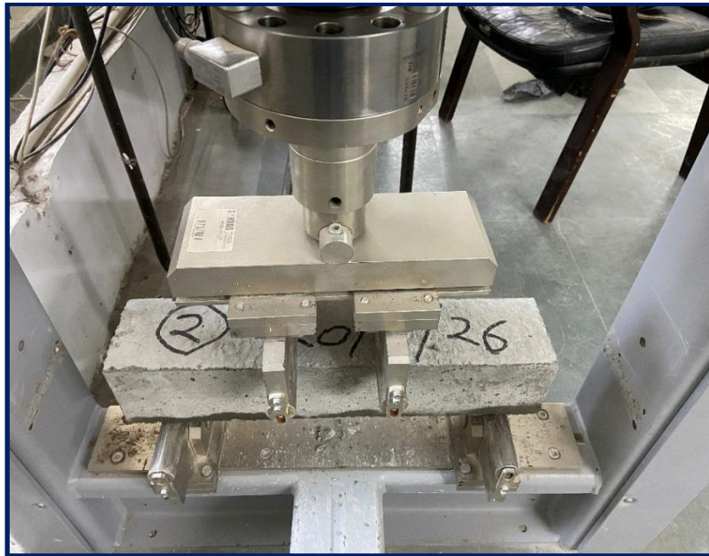
Fig. 6: A typical view of Flexural Strength Test in progress
