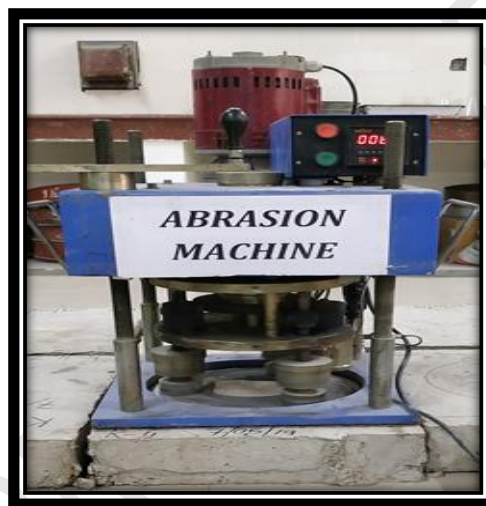
Fig. 9: Horizontal Concrete Slab under Abrasion Resistance Test
