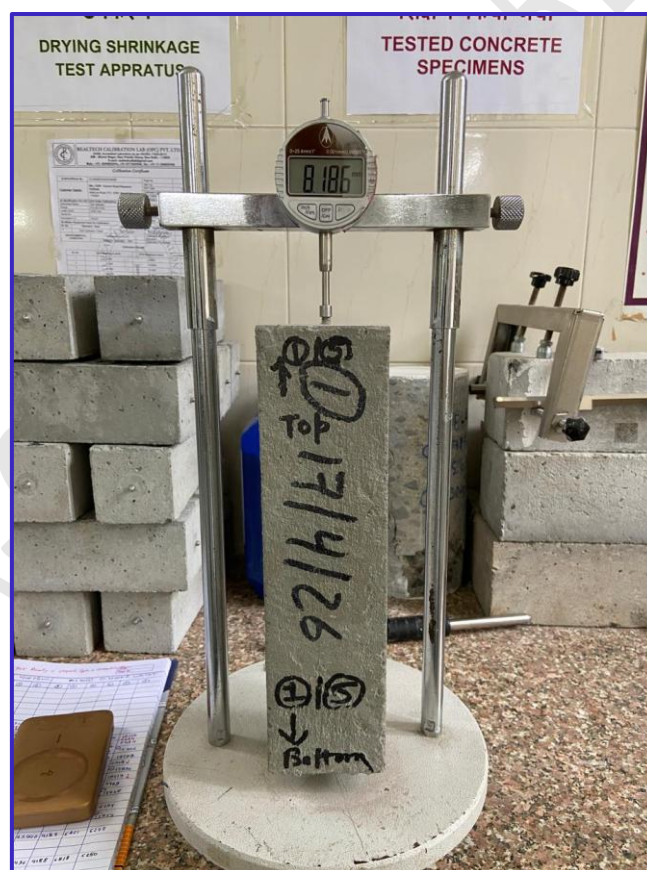
Fig. 12: A typical view of Drying Shrinkage Test in progress
