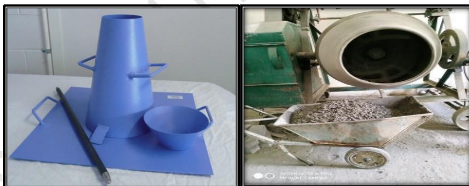
Fig. 2: A typical view of Concrete Mix and Slump Test in progress
