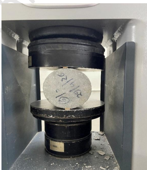
Fig. 8: A typical view of Split Tensile Strength Test in progress
