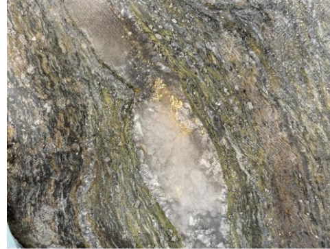
Photo: Visible gold within a boudin of quartz-carbonate vein at 331.4m in NGGRCDD1184
