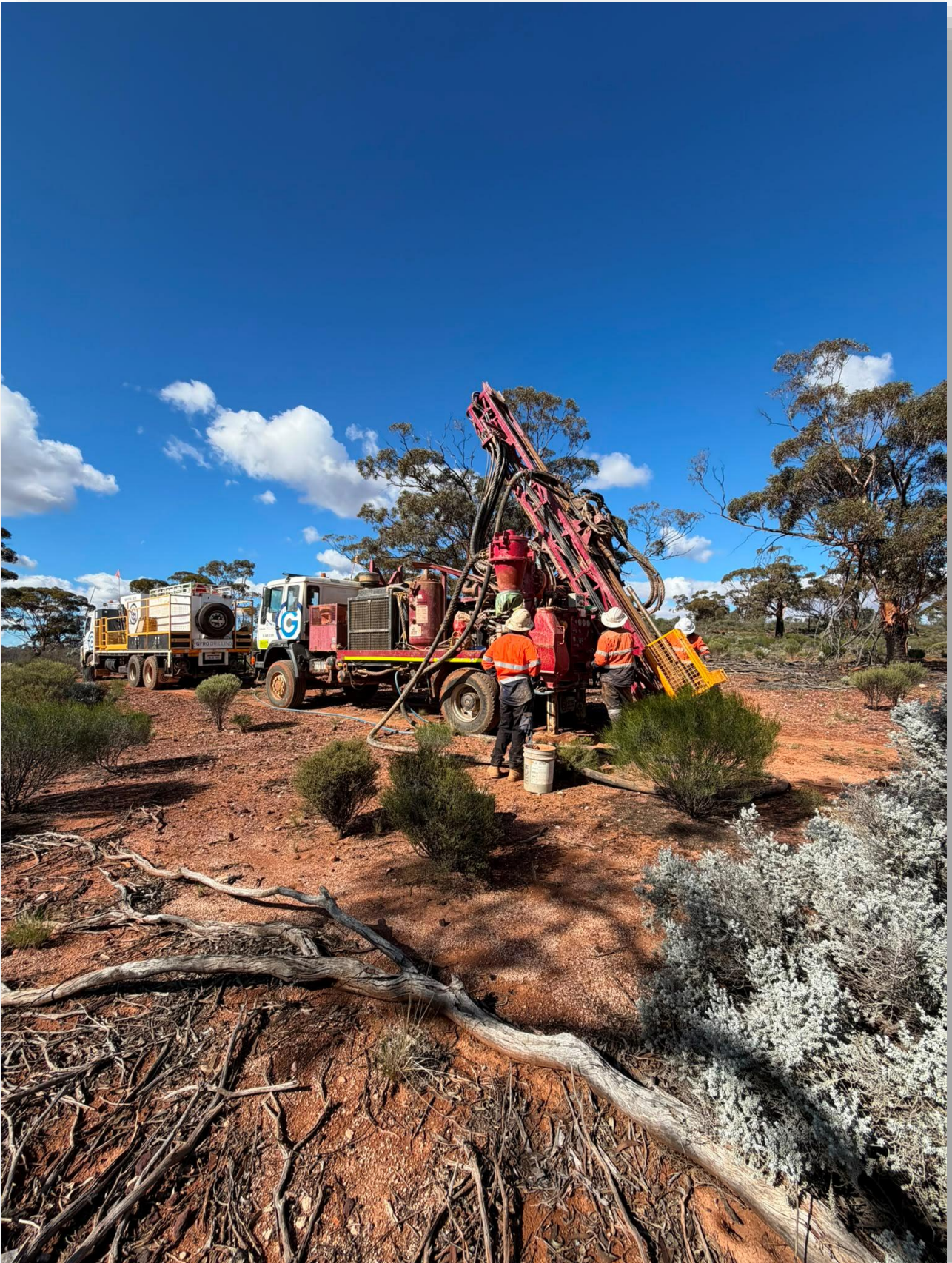
Figure 1: Aircore drilling in progress at the Duchess of York Prospect, Mt Monger Gold Project.
