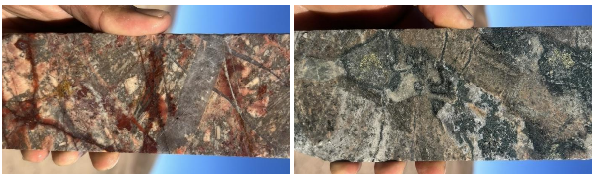
Figure 4: Core photos from CANDD003 showing breccias within the oxide zone with disseminated chalcocite (black) at 134m (LHS) – Breccia within the sulphide zone showing potassic alteration, chlorite muscovite veins with disseminated chalcopyrite at 382m (RHS).
