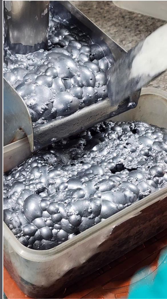
Floatation Testwork on Maronan Silver Lead samples being conducted at AMML Lab in Gosford
