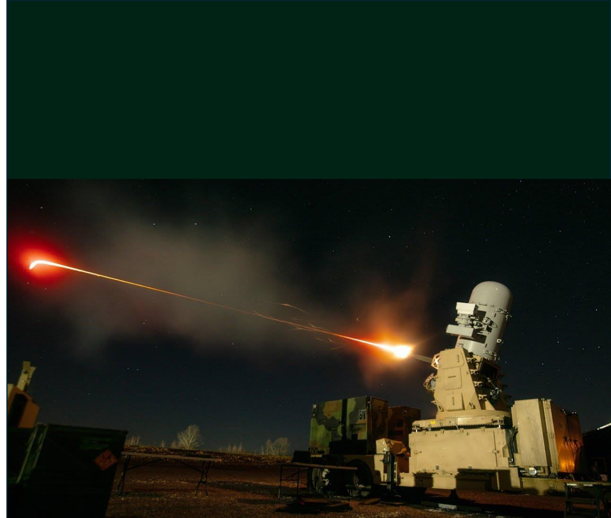
US C-RAM (Counter Rocket, Artillery and Mortar) system firing 20mm (strontium) tracer rounds at a rate of 4,500 rounds per minute
