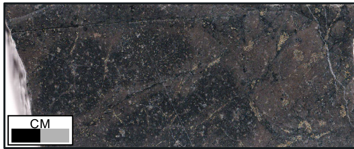
Figure 6: SPD078 – 114.5m, 1.27g/t Au . Disseminated and fracture fill pyrite in a sodic altered andesite with overprinting carbonate veinlets.
