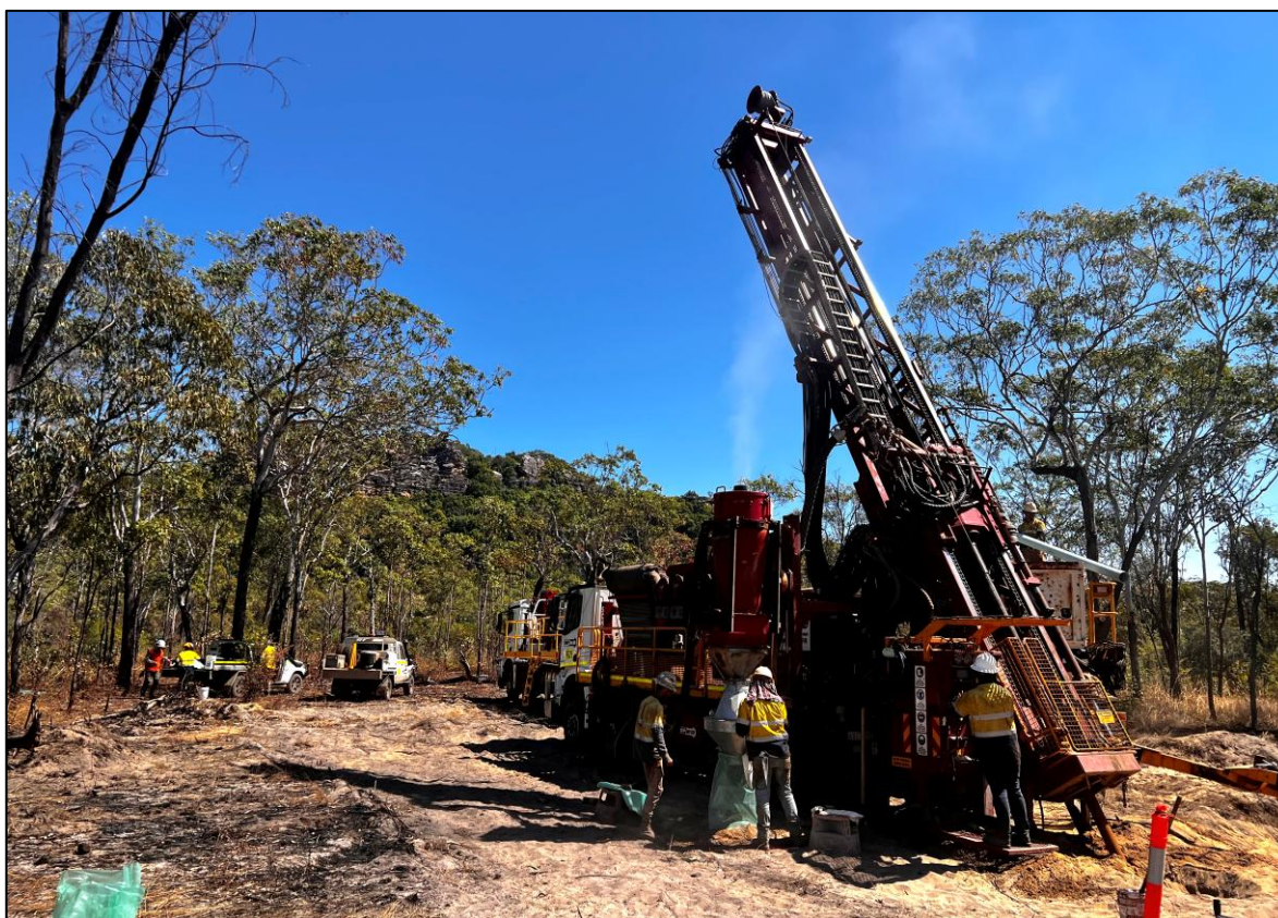
Figure 1: RC drilling underway at the Nabarlek Uranium Project, Northern Territory.
