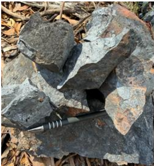
Figure 9: High-grade massive black manganese oxide mineralisation, from mine dump at the Doherty Mine 44.8% Mn, Sample GRR303.
