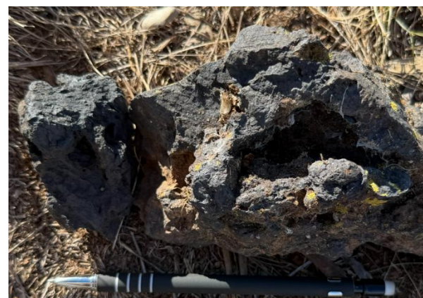
Figure 7: High-grade massive black manganese oxide mineralisation, 49.9% Mn, floater, Sample GRR297.
