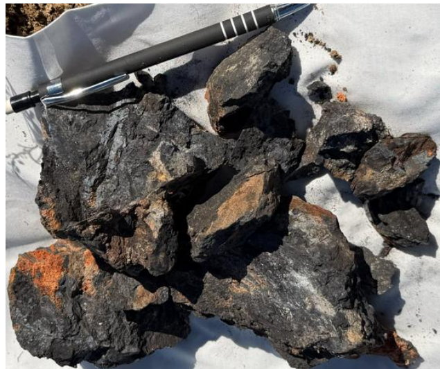
Figure 4: High-grade massive black manganese oxide mineralisation, 46.8% Mn, floater, Sample GRR294.
