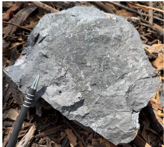
Figure 10: High-grade massive black manganese oxide mineralisation, from mine dump at the Doherty Mine 45.8% Mn, Sample GRR304.
