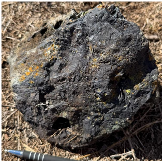
Figure 3: High-grade massive black manganese oxide mineralisation, 51.9% Mn, floater, Sample GRR293.
