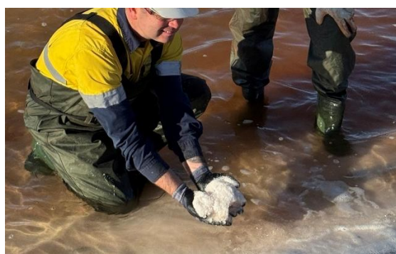
Figure 1: Salt growth in crystallisers
