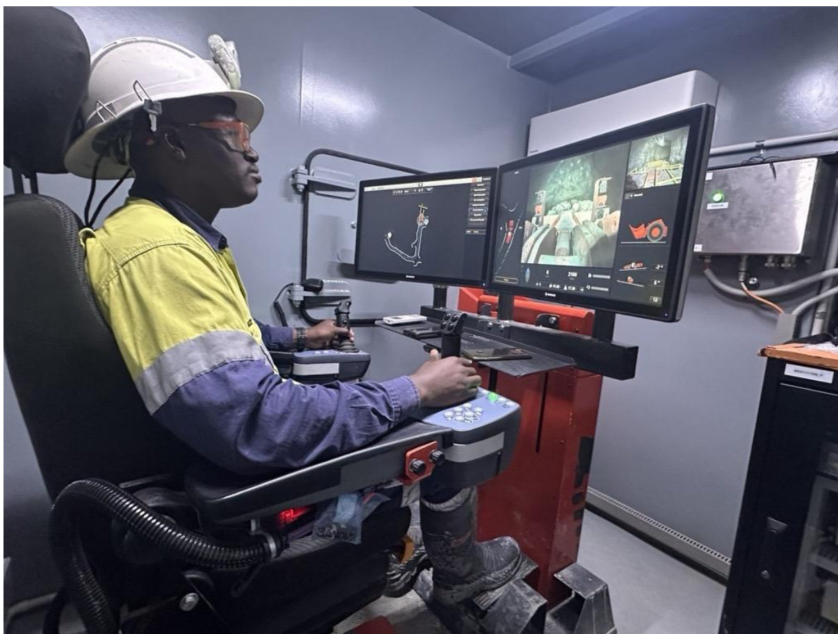
Figure 3: Tele-remote bogging operations at CMA underground
