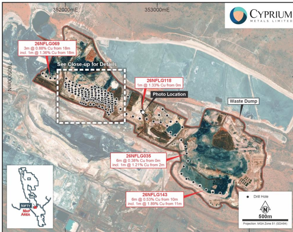
Figure 3: Nifty waste dump drilling locations and scout holes
