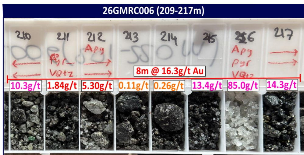
Figure 2: RC chip tray of hole 26GMRC006 (209m - 217m downhole) showing broad intersection of 8m @ 16.3 g/t Au with individual gold grades (to 85.0 g/t Au) shown underneath.
