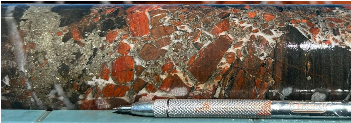
Figure 1: MD002DD HQ core ~524.30 to ~524.50m. Hydrothermal breccia with clotty massive sulphide (15% pyrite, 0.5% pyrrhotite) overprinting earlier formed sheeted quartz veins (left of figure). Cautionary Statement: Visual estimates of mineral abundance should never be considered a proxy or substitute for laboratory analyses where concentrations or grades are the factor of principal economic interest. Visual estimates also potentially provide no information regarding impurities or deleterious physical properties relevant to valuations. The expected timing of assay results is presently unknown.
