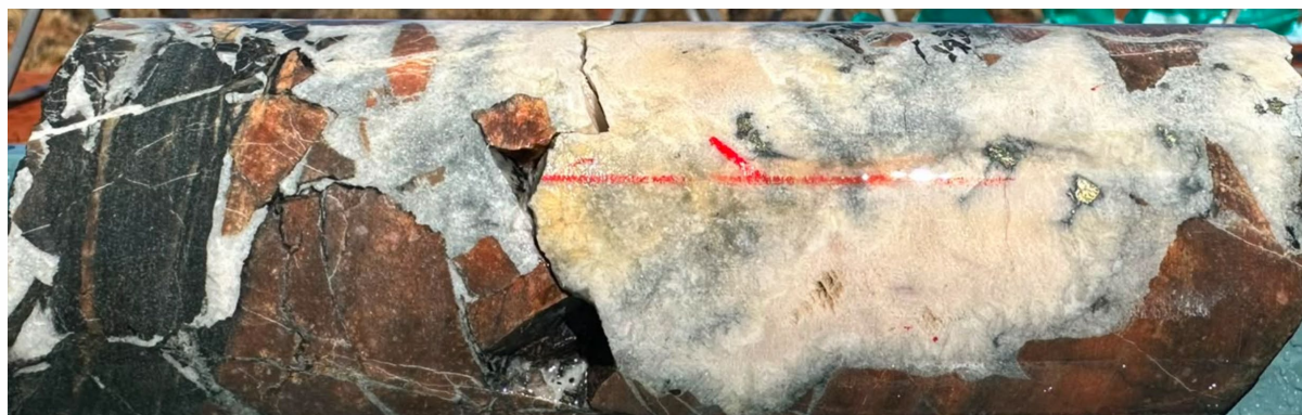
Figure 2: MD002DD HQ core ~521.10 to ~521.20m. Hydrothermal vein breccia with disseminated sulphides (0.25% chalcopyrite, 0.1% pyrite, dark selvage is an unidentified mineral). Cautionary Statement: Visual estimates of mineral abundance should never be considered a proxy or substitute for laboratory analyses where concentrations or grades are the factor of principal economic interest. Visual estimates also potentially provide no information regarding impurities or deleterious physical properties relevant to valuations. The expected timing of assay results is presently unknown.
