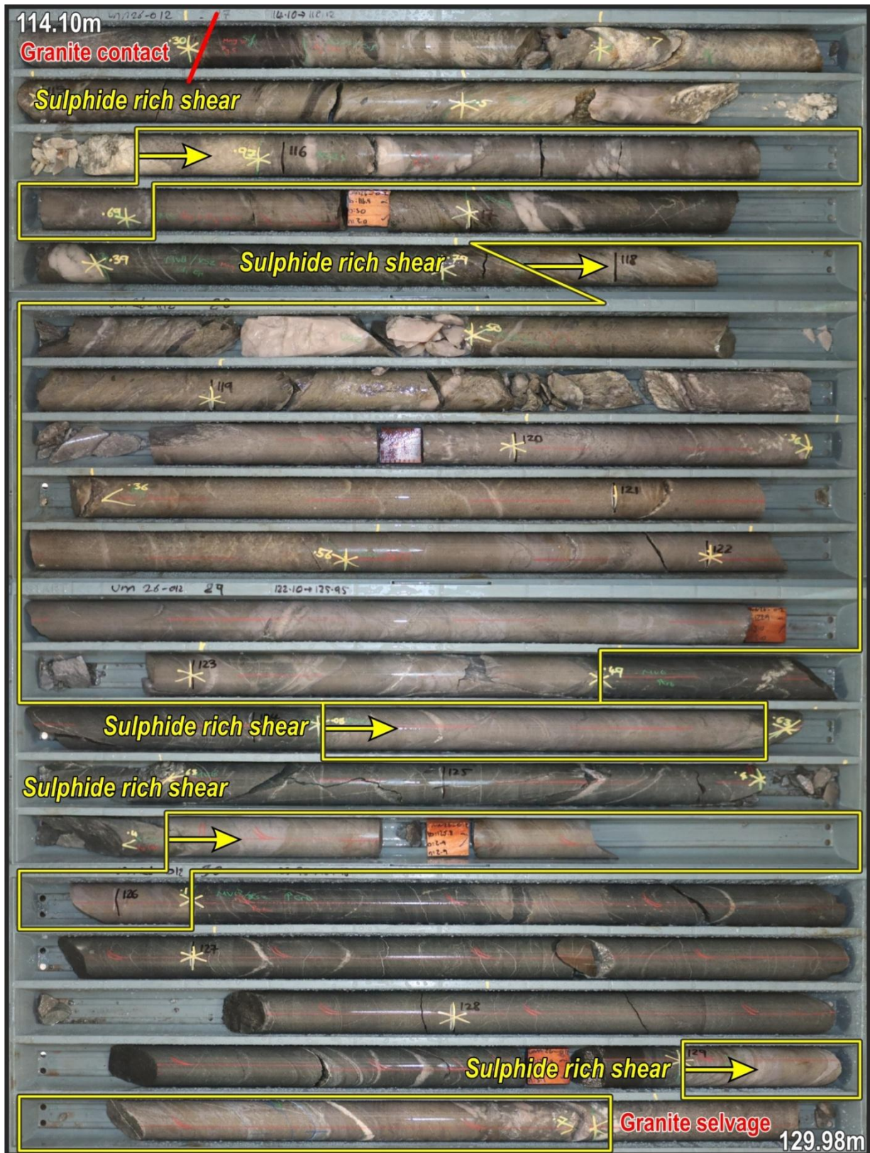
Figure 4 – United North underground diamond drill hole UNN26_012 logged shear (assays pending)*
