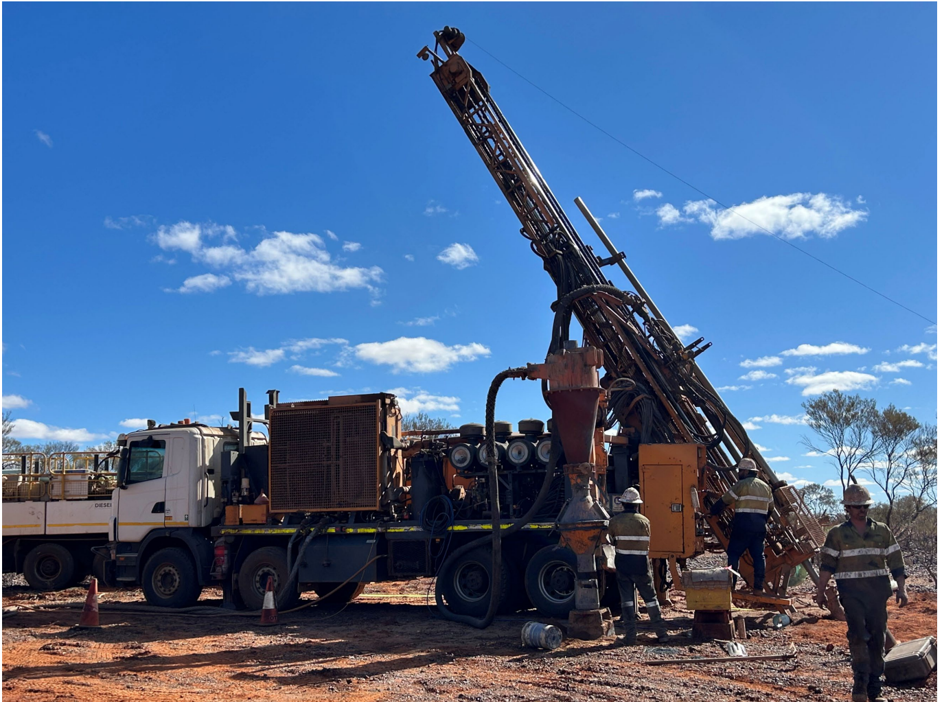
Figure 2: RC Drilling in action testing one of the six copper-gold targets at Juggernaut.
