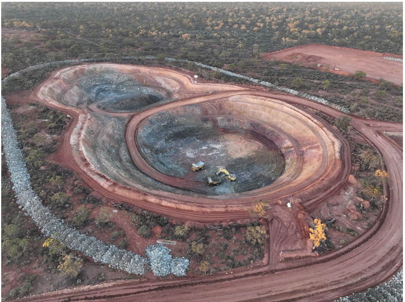
Figure 1: Lady Herial Open Pit - end of June 2026 – the abandonment bund is visible surrounding the pit and is 80% complete.
