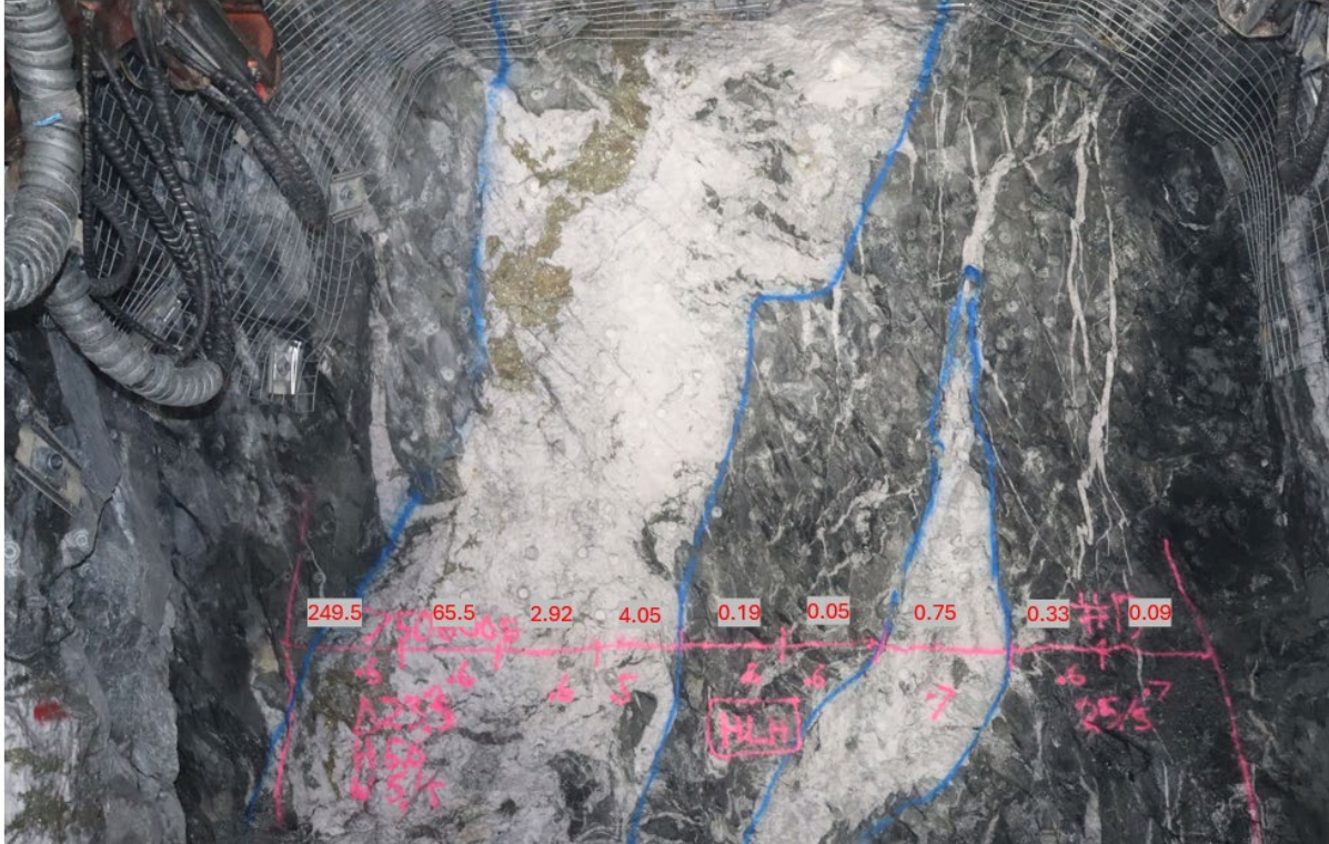
Figure 4: Representative face of Regulus at the 750 level (750_JOD_600_E_13). looking towards mine grid 92 degrees. Face dimensions are 5.00m H x 5.00m W. Area weighted average cut grade 6.28g/t Au.
