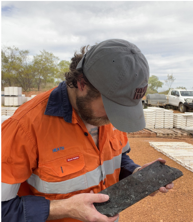
Figure 1 - Core sampling activities at the Halls Creek Project exploration facility. Note: core pictured (left) is from a previously assayed interval in drill hole AORD005; 0.5 m at 35.1% Zn, 20.9% Pb and 546 g/t Ag from 138 m within a broader interval comprising 62.8 m at 1.7% Cu, 18.4% Zn, 4.2% Pb and 99 g/t Ag from 80 m.
