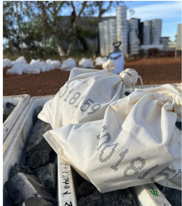
Figure 1 - Core sampling activities at the Halls Creek Project exploration facility. Note: core pictured (left) is from a previously assayed interval in drill hole AORD005; 0.5 m at 35.1% Zn, 20.9% Pb and 546 g/t Ag from 138 m within a broader interval comprising 62.8 m at 1.7% Cu, 18.4% Zn, 4.2% Pb and 99 g/t Ag from 80 m.
