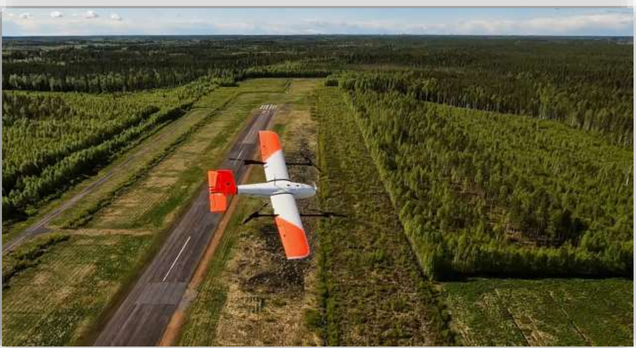
Figure 2. Radai drone used to collect high-resolution magnetic and radiometric data.
