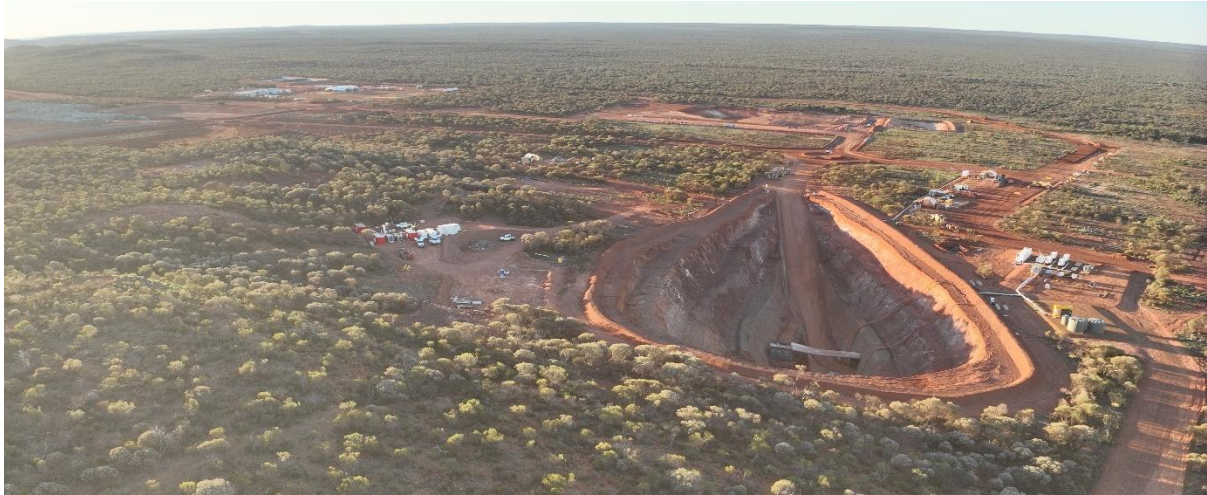
Figure 5: Gossan Valley box cut and decline development - looking north-east
