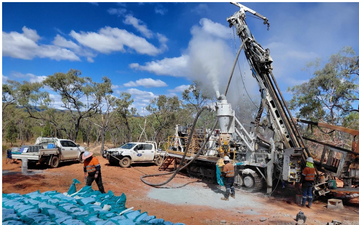
Figure 2 Tracked-mounted RC rig drilling at Orient (Drill Hole ORR209)
