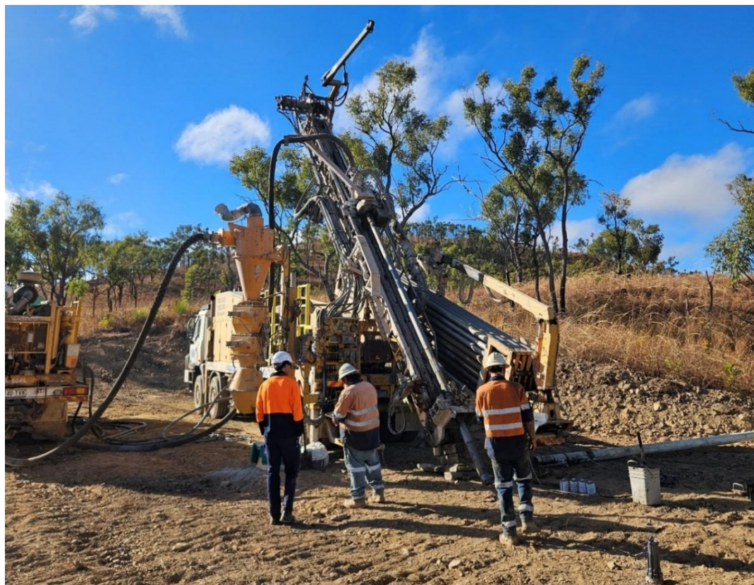
Figure 1 Wheel-mounted RC rig drilling at Boonmoo Epithermal (Au-Ag) Target (Drill Hole BERCO03)
